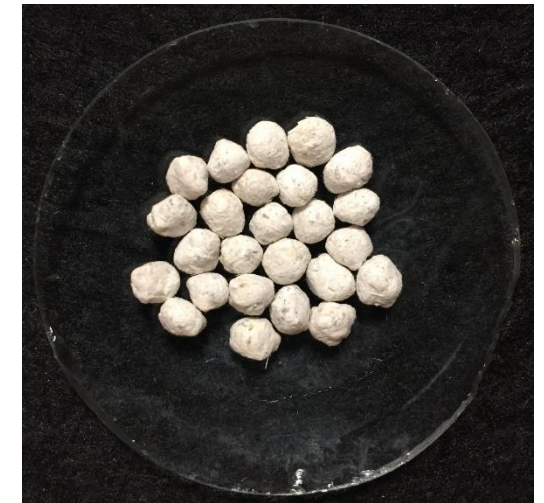
Fertiliser with keratin-based coating prepared at lab scale in KaRMA2020
