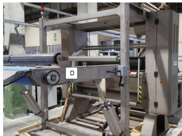
R2R sonochemical fabric coating machine for hospital textiles at Klopman
