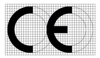
If the CE marking is reduced or enlarged, the proportions given in the graduated drawing shall be respected. However, the CE marking shall be at least 5 mm high.
